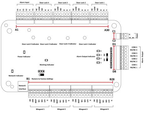
Figure 3-3 DS-K2804 Access Controller Terminals
