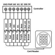
Figure 4-1 Wiring diagram of Wiegand card reader
