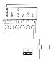
Figure 4-4 Wiring diagram of anode lock
