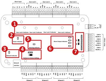
Figure 2-1 DS-K2804 Component Schematic Diagram
