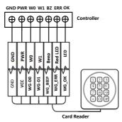
Figure 4-2 Wiring diagram of 1800 series card reader
