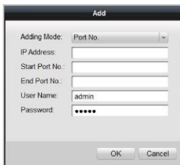
Figure 8-10 Adding by Port No.
