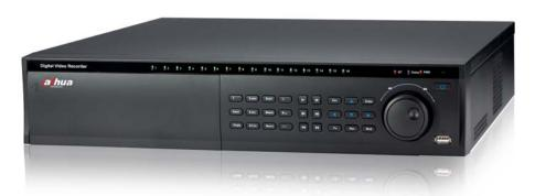
DH-DVR0804LE-S: 8 channel video inputs, 8 channel audio inputs, 8 channel loop outputs and 1 channel matrix output. The 1st video channel can support max D1(4CIF) realtime recording and other channels can support CIF realtime recording. It can support VGA, HDMI, eSATA, USB2.0 and 4 HDDs.
