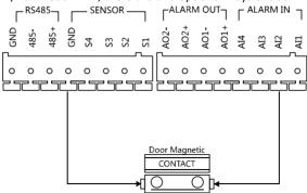
Figure 3-17 Door Magnetic Wiring for DS-KD8102-V/DS-KD8002-VM (1)
