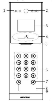
Figure 1-4 Front Panel Keys
