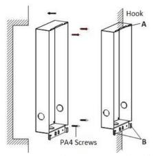
Figure 3-9 Insert the Gang Box into the Wall
