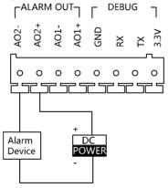
Figure 3-27 Alarm Device Output Wiring for DS-KD6002-VM
