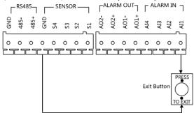
Figure 3-20 Exit Button Wiring for DS-KD8102-V/DS-KD8002-VM (1)
