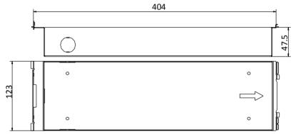
Figure 3-1 Front and Side View
