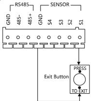
Figure 3-21 Exit Button Wiring for DS-KD8102-V/DS-KD8002-VM (2)
