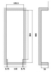
Figure 3-8 Dimensions of the Hole
