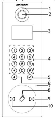
Figure 1-1 Front Panel Keys
