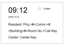
Figure 6-3 Main Interface of Outer Door Station
