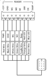
Figure 3-23 External Card Reader Wiring
