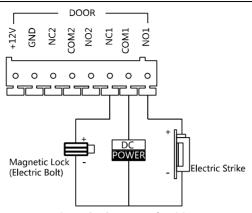
Figure 3-16 Door Lock Wiring
