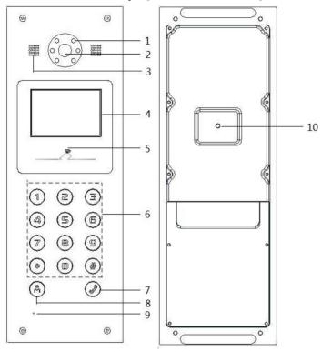
Figure 1-6 Front Panel Keys and Rear Panel Keys
