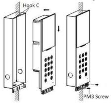
Figure 3-10 Install the Door Station
