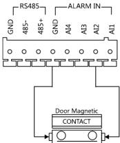
Figure 3-19 Door Magnetic Wiring for DS-KD6002-VM
