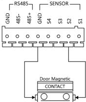
Figure 3-18 Door Magnetic Wiring for DS-KD8102-V/DS-KD8002-VM (2)
