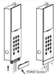
Figure 3-11 Secure the Door Station
