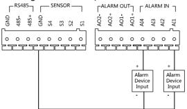
Figure 3-24 Alarm Device Input Wiring for DS-KD8102-V/DS-KD8002-VM
