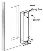
Figure 3-3 Insert the Gang Box into the Wall
