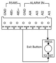
Figure 3-22 Exit Button Wiring for DS-KD6002-VM
