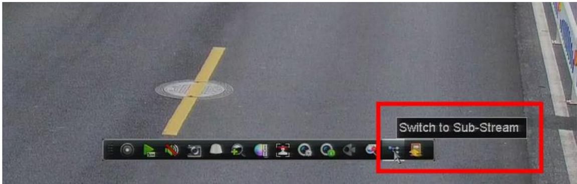
(2) User can set default live view stream type in Configuration-Live View-View-More Setting, supported modes include Main Stream, Sub Stream, Auto. Reentering the live view interface or switching live view spilt-screen mode will turn to default live view stream type.
